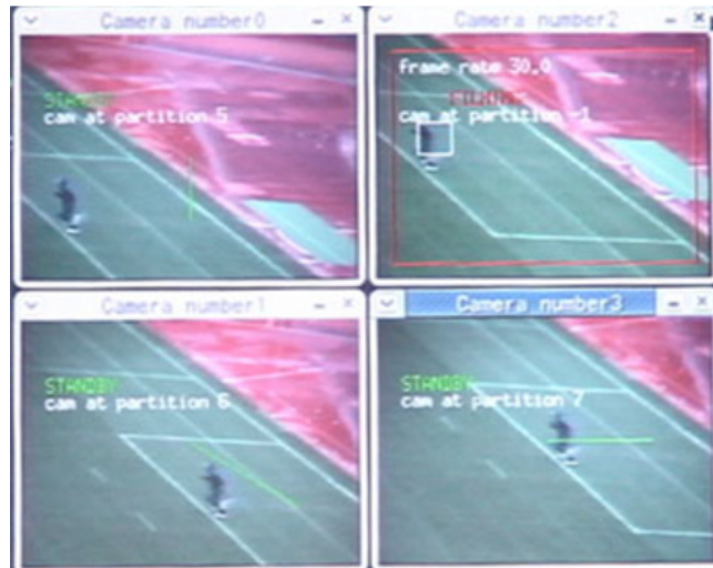
Figure 6: Tracking result 1, each of stand-by-cameras take a position and wait for the target
