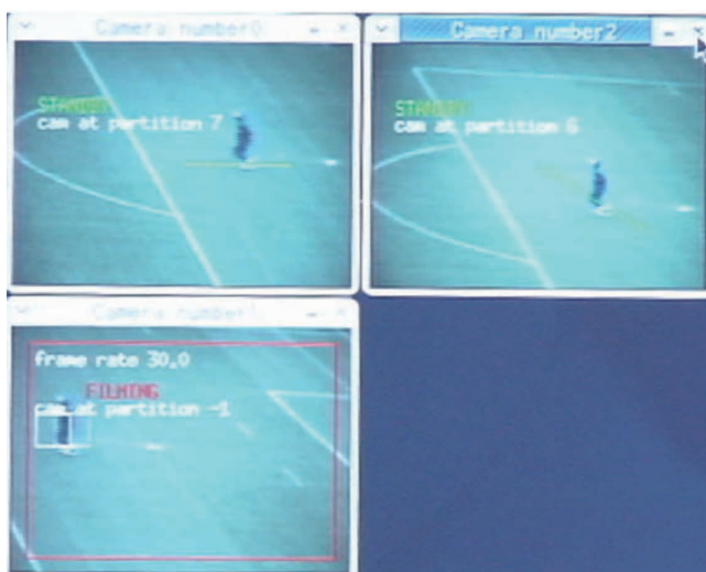
Figure 10 Tracking result 2 using 3 cameras; while the monitoring camera is filming the object, each of the stand-by cameras takes a position and waits for the target
