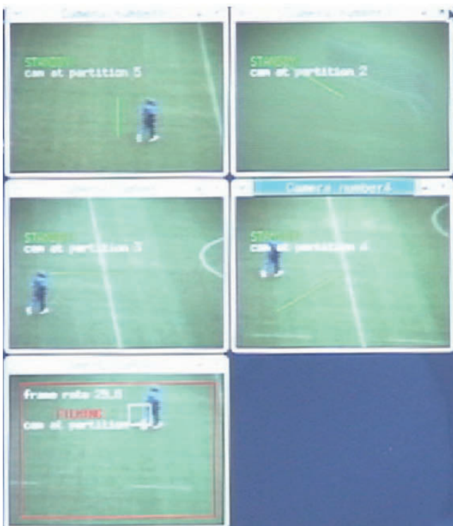
Figure 11 Tracking result 1 using 5 cameras; while the monitoring camera is filming the object, each of the stand-by cameras takes a position and waits for the target
