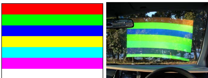
Figure 6 – Experiment to show colors on the WHUD. Colors except for green are faint due to the material comprising the windshield.
