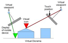
Fig. 3 Input method of attention point by Virtual Diorama. Users can input an attention point on a miniature 3D CG model. Our system shows visual icons with different colors for each user at the attention point.
