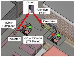
Fig. 1 Concept of Virtual Diorama. Users can observe a miniature CG model of real world around themselves through mobile handheld device's monitor.
