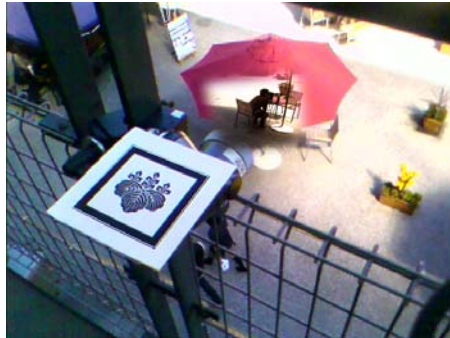
Fig. 7 Snapshot image of See-Through Vision. User can observe invisible space using the images from environmental cameras.
