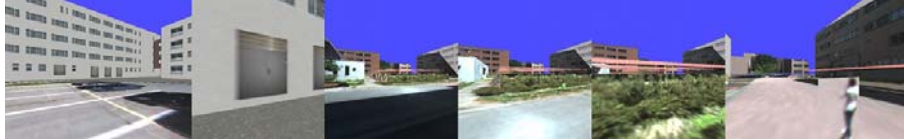
Fig. 5 Example of virtual viewpoint motion. A user's viewpoint comes through the building in front of him/her (left to right).
