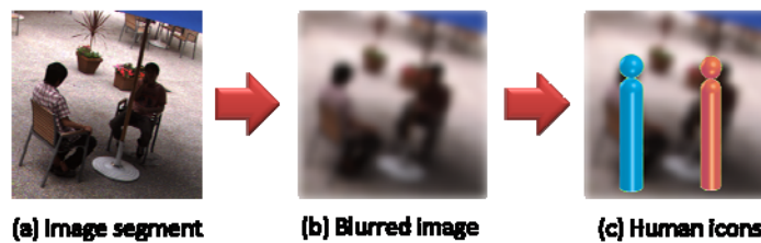
Fig. 8 Privacy-safe visualization. (a) An image segment captured by a surveillance camera. (b) Blurred image making recognition impossible. (c) Human-shaped icons.
