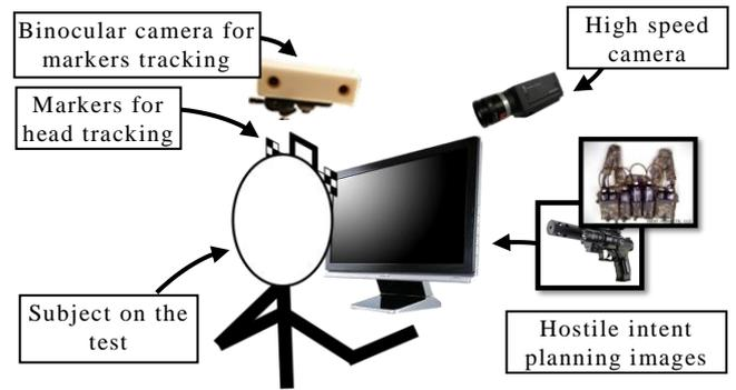
Figure 8: Illustration of experimental setup, where the subject is interviewed by computer about his hostile action planning using special images. For recording subject facial motions high speed camera is used. Binocular camera is used for extracting the 3D location of the face by tracing special markers that are attached to subject head.
