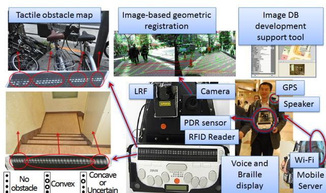
Figure 1. Overview of indoor-outdoor navigation system for visually-impaired pedestrians.
