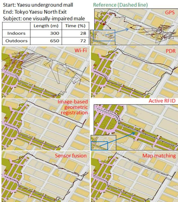
Figure 3. Overview of trajectories obtained with each sensor and method.
