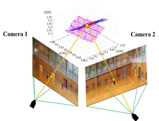
Fig. 1. 3D Trajectory estimation of badminton shuttle using Shape-From-Silhouette technique.
