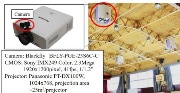
Figure 1. Large scale projection-based AR system in a gymnasium
